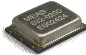
**The Model 832M1** is a low cost, board mountable triaxial accelerometer. Featuring stable piezo-ceramic crystals, the accelerometer incorporates full power and signal conditioning with a maximum current consumption of 22 micro-amps. The model 832M1 is available in  $\pm 25g$  to  $\pm 500g$  ranges and provides a flat frequency response up to greater than 6kHz. The standard model 832 offers the same envelope with a lower maximum current consumption of 4 micro-amps.
